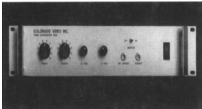
Model 310A video integrator from Colorado Video.
