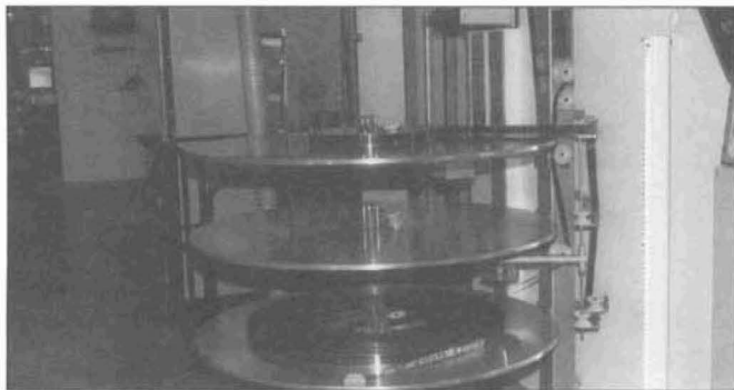
The feeder elevator system at Stockholm's Filmstaden Sergel.
