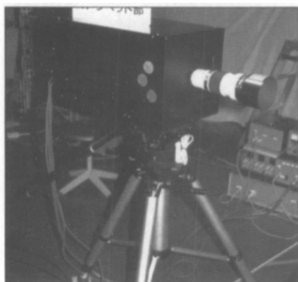
Figure VC-4. The 4K x 2K pixel progressive color scan camera system from NHK.
