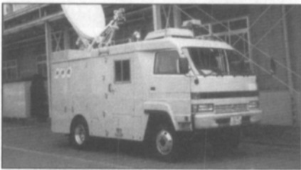
Figure TS-3. Hi-Vision communication satellite transmission system from NHK.
