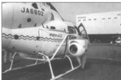
Figure NG-2. NTS's HDTV helicopter camera system.
