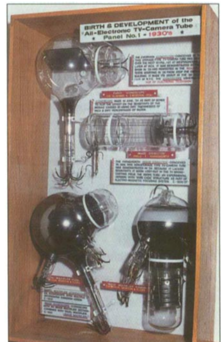
Fig. TM 1. A display of early developmental imaging tubes. From top: Zworykin's Iconoscope (ca. 1934), Farnsworth's Image Dissector (ca. 1930-31) and a pair of later Zworykin-Morto-Flory Iconoscopes with multiplier stages (ca. 1937). Photo courtesy of Manhattan College.
