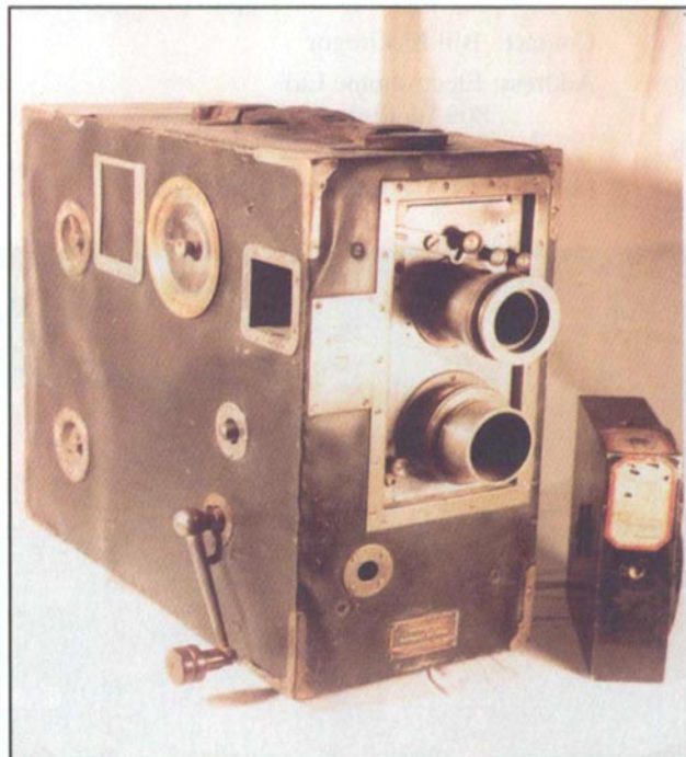
Fig. AKC 1. Professional 35mm camera made by Bell & Howell, #5, ca. 1909. It had a wooden body and was soon superseded by the better known model 2709. One of only three currently known existing examples.
