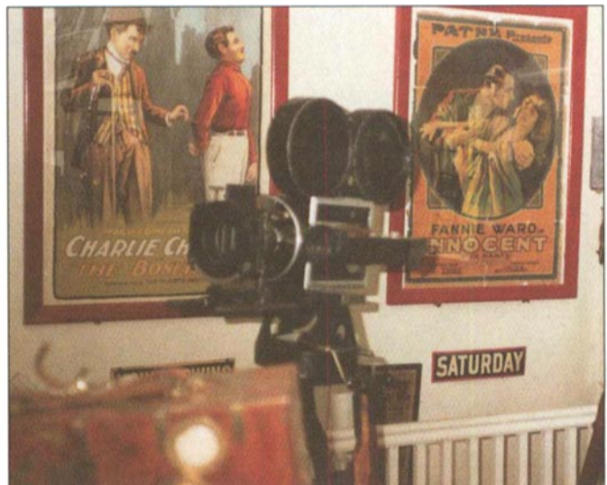
Fig. MCS 2. 1939 Art Deco Brenkert projector with RCA soundhead as shown at the 1939-40 San Francisco World's Fair.
