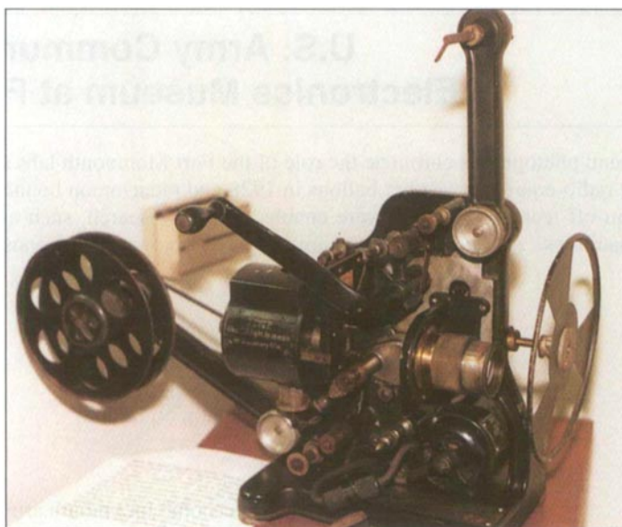
Fig. VRC 1. Patheoscope itinerant projector, ca. 1920. The machine is equipped with a hand crank and a sewing machine motor which allowed the projectionist to adapt to whatever facilities he encountered. It is assumed he carried a storage battery to light the lamp if no electricity was available. The width of the film is about 32mm.
