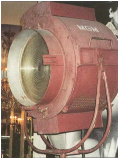
Fig. M. 1. Mole-Richardson 5-kW "Brute" high-intensity carbon arc spot lamp with 24-in. diameter lens used at MGM studios in the 1940s and 50s. Photo courtesy of Debbie Reynolds Museum.
