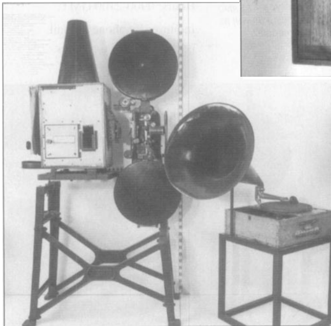
Fig. DM 4. In 1903, Oskar Messter, the German film pioneer, introduced his Biophon sound-on-disc device. Projector and gramophone were driven by electric motors and made to coincide by a synchronizing mechanism. Photo courtesy of Deutsches Museum, München.
