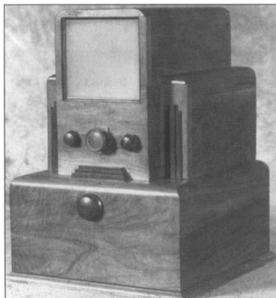
Fig. MST 2. Scanning disc television (1932), built in Montreal to receive some of the first television broadcasts in Canada. Photo courtesy of National Museum of Science and Technology Corp.
