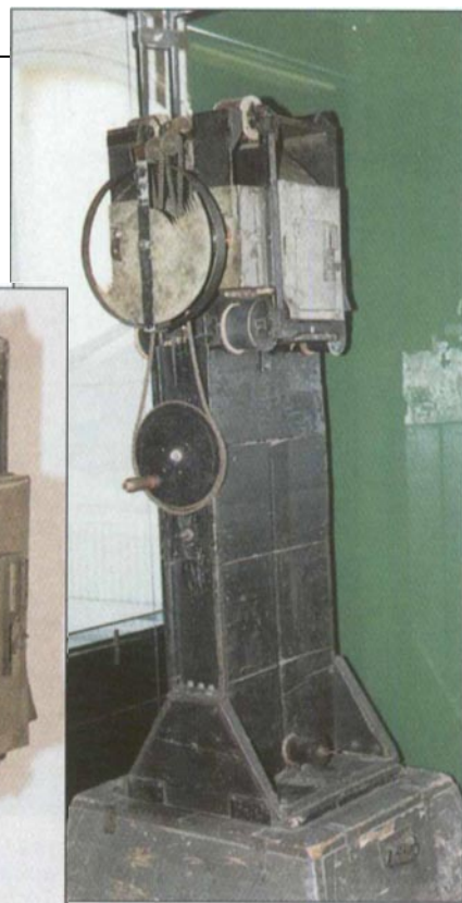
Fig. FMP 1. The Bioskop projector by Max Skladanowsky (1895) is a dual-head projector designed for alternate projection of two strips of film at a rate of 16 frames/sec. Photo courtesy of Film Museum, Potsdam.
