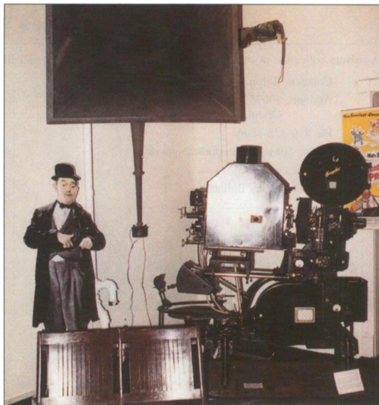
Fig. CWC 1. Clockwise from top: Ultraphone speaker horn of 1928 from Standard Theater, Chicago; Super Simplex projector head on Western Electric base for sound-on-film and on disk with variable speed turntable, 1928 (the projector head has a turret for a Magnescope lens and uses a high-intensity condenser carbon arc lamp by Hall and Conelly); outdoor folding chairs from the Mosholu Theater, a rooftop theater in the Bronx, NY, 1926.
