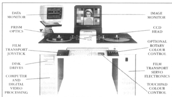
Figure 1: The once manual procedure of grading is now done with the aid of sophisticated electronic equipment linked with computers.
