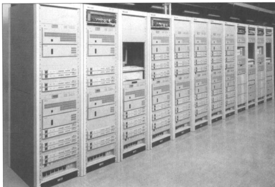
Fig. NHK 1. A large scale still picture system with video servers.
