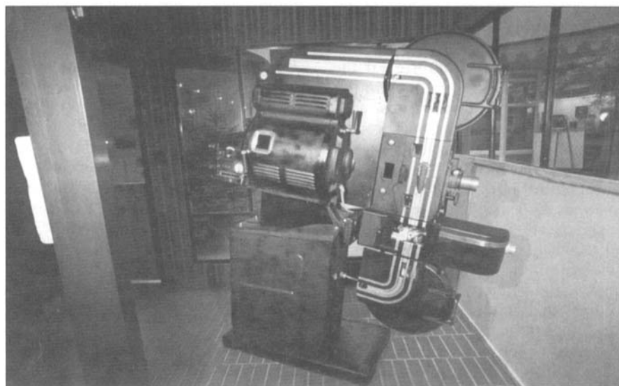
Fig. MCS 2. 1939 Art Deco Brenkert projector with RCA soundhead as shown at the 1939-40 San Francisco World's Fair.
