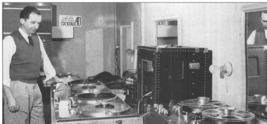
Jack Mullin, in 1949, with his two portable Ampex Model 200 audiotape machines. The model 300 is pictured in the foreground.
