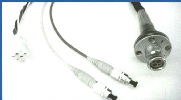
Nemal's fiber-optic patch panel for SMPTE standard connectors.
