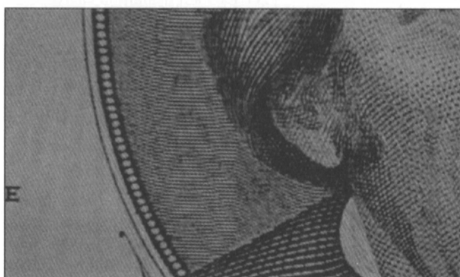
Figure 9. Interlace HDTV: frame freeze, close-up of $20 bill engraving.
