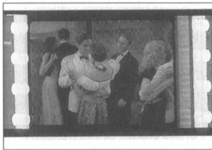
Combined picture and sound 'lavender' inter-positive print. Although looking like a rather dense release print, its purpose was for making duplicate negatives. Note the Bell & Howell negative perforations.
