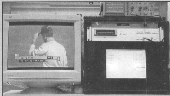
The msi2080 8VSB reference receiver from Modulation Sciences
