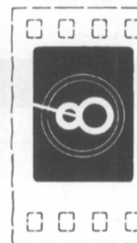
Figure 2 — 16-mm sound start identification frame
