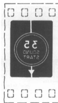
Figure 3 — 35-mm sound start identification frame
