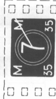
Figure 3 — 35-mm sound start identification frame
