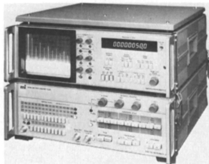
An automatic white noise test set, Model 2090C, and a spectrum analyzer, Model 2370, shown above, have been announced by Marconi Instruments Ltd., Longacres, St. Albans, Hertfordshire, England, represented in the United States by Marconi Electronics Inc., 100 Stonehurst Court, North Vale, NJ 07647. The 2090C
