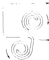
Fig. 11. Principle of the bi-filar winding used in the Loopmatic: the continuous loop of film is wound as a double spiral on each spool in turn.
