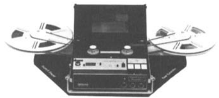
Optional Reel Extenders increase the 19-minute running time of Super8 Sound Recorder I to one hour.
