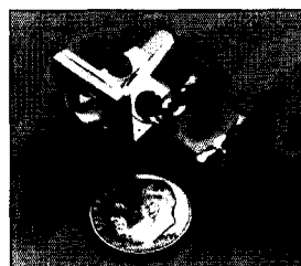
Miniature solar cell permanently fused to light-gathering prism. Coherent light beam for clean sound, less ambient light "noise."
