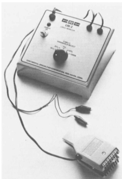
A 16-channel clip-on Logic Monitor, Model LM-1, for testing a digital dual in-line plug (DIP) has been announced by Continental Specialties Corp., 44 Kendall St., P.O. Box 1942, New Haven, CT 06509. An LED at each pin indicates the state of that pin by lighting or remaining dark. By monitoring an entire 14- or 16-pin DIP at once, the logic monitor reveals the action of the package as a whole. Model LM-1 tests DTL, TTL, HTL and CMOS logic families. It automatically seeks out the highest positive and lowest negative voltage levels and draws its power from the IC under test. Individual comparators at each pin (100,000 \Omega input impedance) drive individually-labeled LEDs "on" for a high and "off" for a low logic level. The price is about $74.95.
