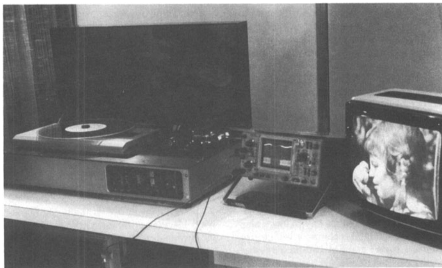
Fig. 5. A notable technical achievement at Montreux was the instant-playback, broadcast-quality color videodisk machine displayed privately by Thomson-CSF. The disk is rigid plastic with a thermally activated layer. Images, recorded and played back by lasers, can be still-framed, time-shifted, or run at normal speeds.
