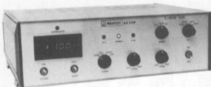
Unique in-line cross-modulation generator and automatic mode-switching reader. RA-1718: Reader alone RA-1719: Generator/Reader
