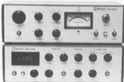
RA-1712 and RA-1713 Completely redesigned transformerless, solid-state recording electronics for updating RCA, Maurer, and older Westrex systems.
