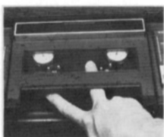
The T2-H15-UM TENTELOMETER® Tape Tension Gage shown checking the critical hold-back tension on a Sony 2850. Price $225 complete.
