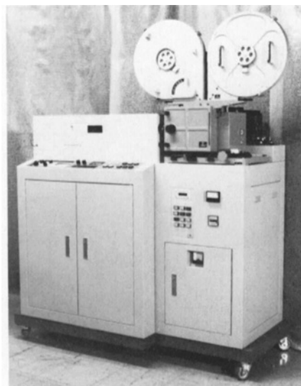
Fig. 1. Overall view of a prototype 16mm laser beam sound recorder.
