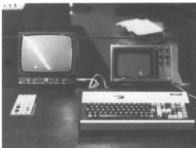
Figure F-2. Cap-Gen electronic character genera- tors used in YLE for titling.
