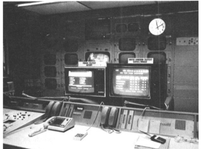
The master control room at KMOX-TV during the teletext testing period. Two additional TV receivers were installed: (left) a Thomson-CSF set working on Antiope, and (right) a Zenith receiver modifier to operate on Ceefax/Oracle.
