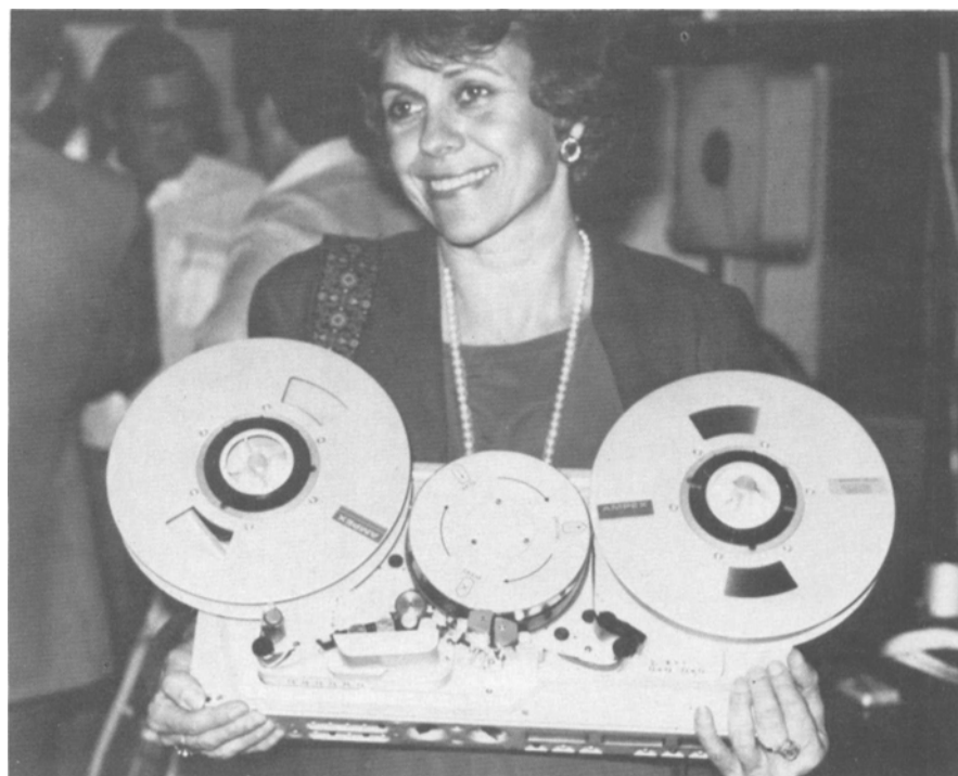
Figure 3. New product hit of the show was the Ampex/Nagra VPR5, 1-in. Type C recorder weighing in at just 15 lb.
