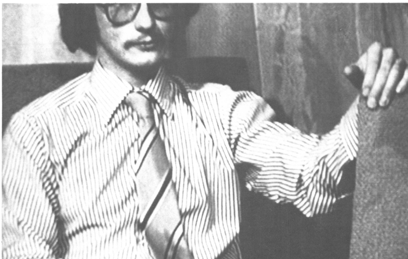
Figure 7. Philips Hi Fi Zero PAL demo produced excellent pictures using a frame store in the PAL receiver to eliminate the usual defects found in such images. This closeup of the screen shows excellent high frequency luminance detail in striped shirt without the familiar cross-color moiré patterns.
