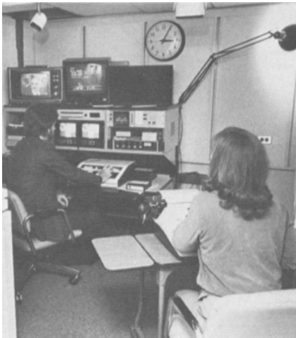
Figure T-3. One of 18 helical recorder editing cubicles in the ABC Washington News Bureau.
