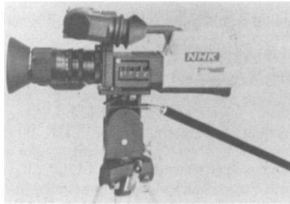
Figure J-13. Single tube color camera (NHK).
