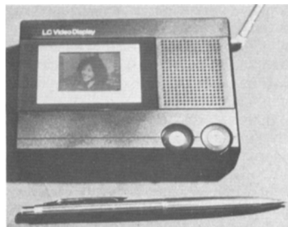
Figure J-24. Liquid crystal video receiver.
