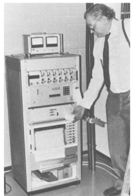
Figure F-5. Vibration of the masts and guys are continuously monitored by automatic logging equipment.
