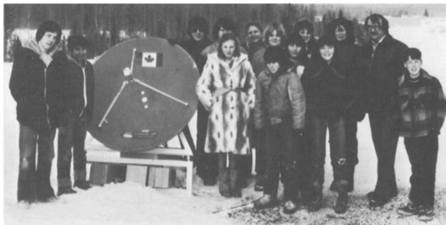
A 1.8-meter TVRO Earth DBS receiving terminal at Beardmore, Ont., Canada.
