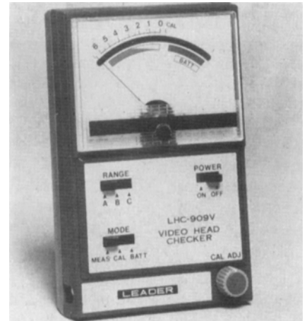
LHC-909 for checking video head wear, Leader Instruments Corp.
