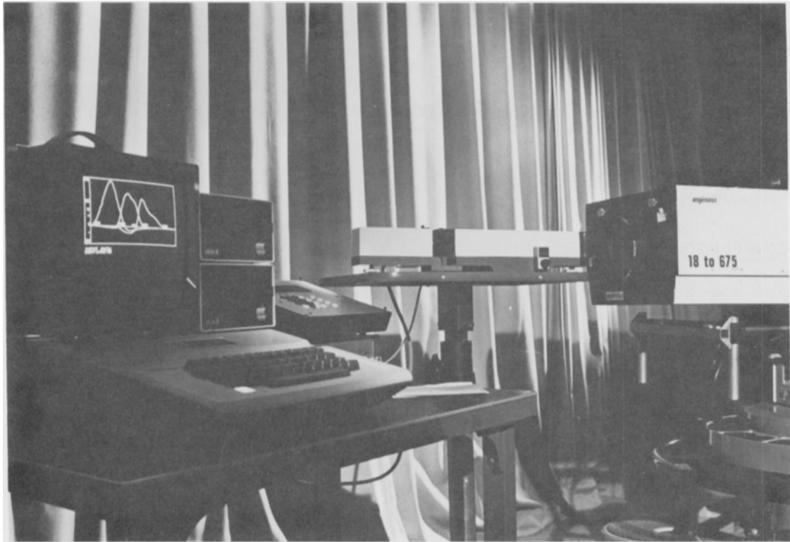
Fig. 1. The picture illustrates the prototype arrangements of the IBA's computer-operated spectrophotometric analysis of cameras equipment.
