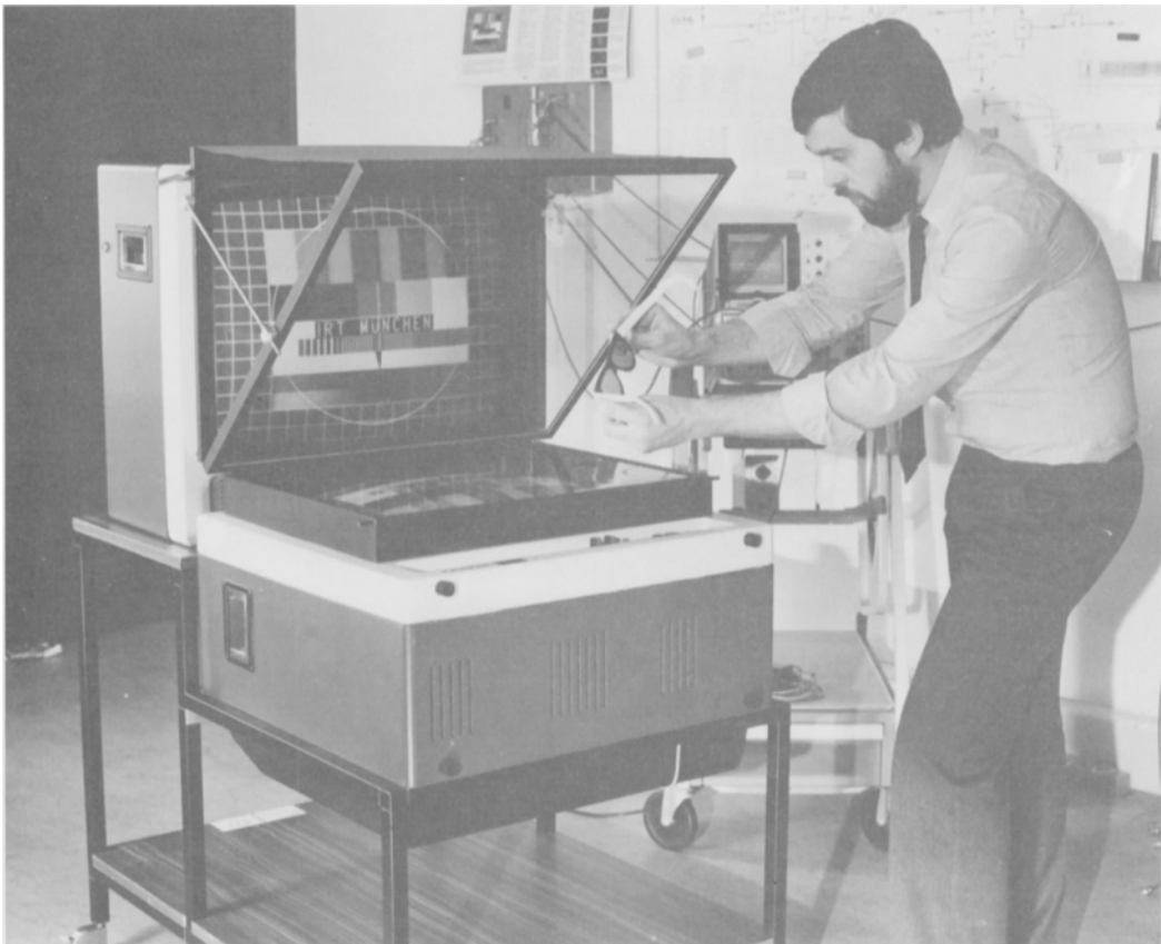
Fig. 6. 3D display device with two 26-in. monitors, polarizing filters and a semi-transparent mirror (IRT).
