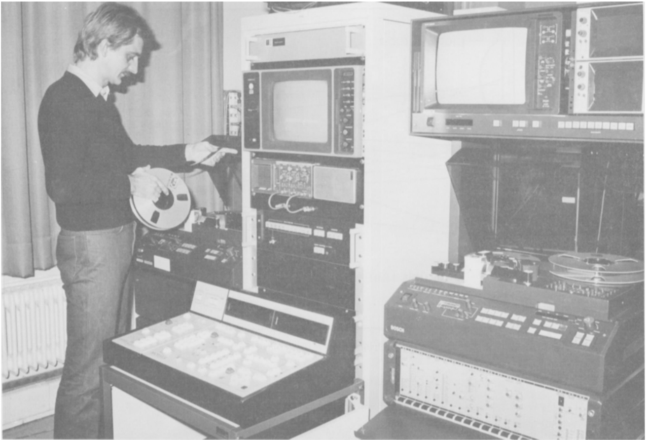
Fig. 5. 3D recording and display equipment consisting of two B-format VTRs (Bosch-Fernseh) and the MOSAIC editing system (IRT).
