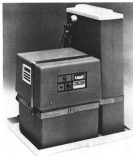
Auto/Plater silver recovery unit, Allen Products Co.
