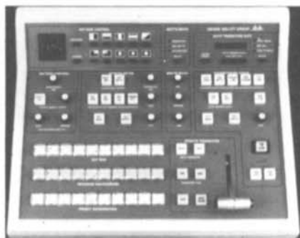
Grass Valley Model 100CV production switcher
