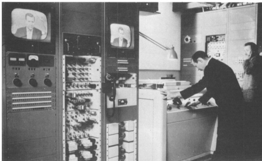
The production version of the first practical VTR used by CBS on November 30, 1956.
