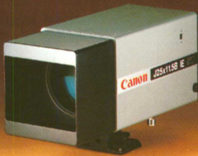
J25x11.5BIE for 2/3" cameras. Greater Reach—a 25X zoom lens designed specifically for 2/3" cameras. The power and scope of 1" systems, the economy and efficiency of your 2/3" cameras. Focal length: 11.5-288mm (23-576mm w/2X extender) Max. Relative Aperture: 1:1.6 through 220mm 1:2.1 at 288mm
