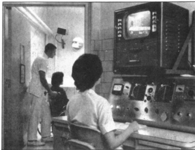
(Left) Dentistry students viewing TV demonstration. Studio is linked to three auditoriums accommodating 150 students each; (Right) One of three installations in Radiation Therapy Center at the Medical School. Vidicon camera, upper left, surveys patient under treatment and is monitored by technician • Television and the University • R. J. Stanley • Journal of the SMPTE , April 1963.
