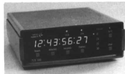
Telcom TCG-550 time-code generator
