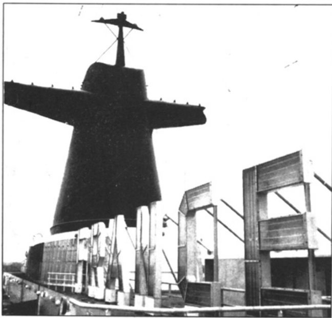
(Left) Aft funnel with three Yagi aerials mounted on a support designed specially for this service by the shipbuilder. (Right) The two H-Q cameras coupled with two 16mm film projectors and two 16mm perforated tape recorders • The Television Installation on Board the S.S. France • P. M. C. van der Spank • JSMPT, July 1963.
