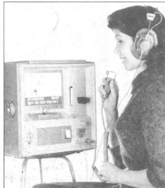
Ligatron during operation using the headset • Self-Contained 8mm Sound Language Teaching Machine • L. H. Schank • JSMPE , September 1963.
