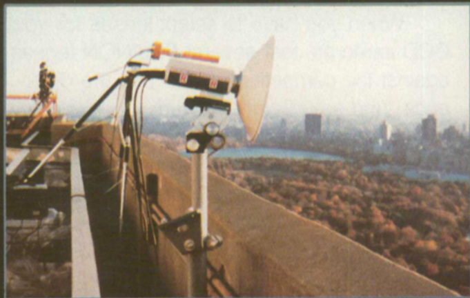
The PP-70 provides coverage from atop the Gulf & Western Building to a receiver at ground level for window-link transmission.
