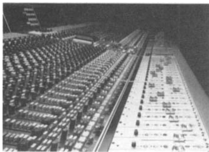
Neve console automation system
