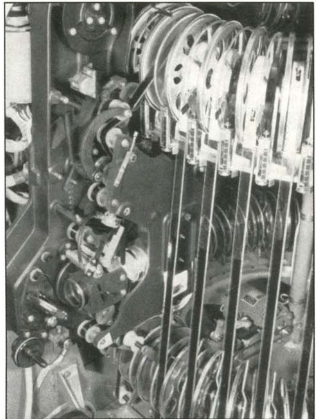
(Left) Projector with threading arm in open position; (Right) Threading arm in projecting position • Preparation and Projection of Multilingual Films • G. W. Tressel and S. J. Andrews, Jr. • JSMPE , December 1965.
