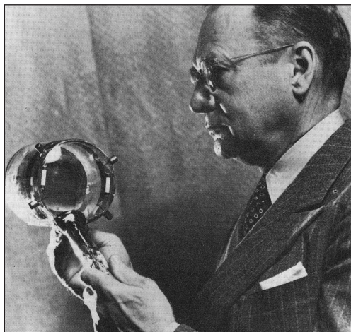
An early model of the iconoscope is shown with its inventor, Dr. V. K. Zworykin. (Photograph courtesy of RCA.)
