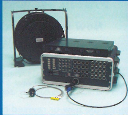
The DTV-4200 4-channel SDI and audio fiber optic transport system from Multidyne.
