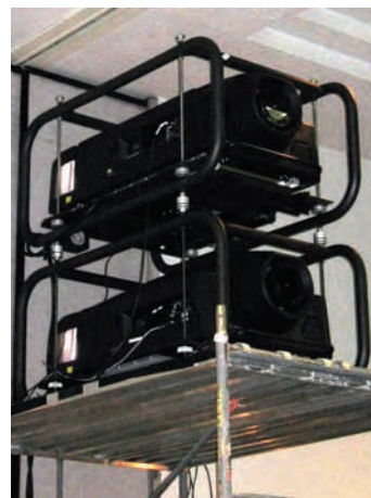
Figure 1. Stacked projectors create co-located pixels for 3-D images.
