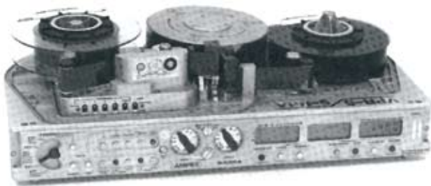
VPR-5 portable Type-C VTR, Ampex/Nagra (Fig. T-3 from SMPTE Journal April 1984, p. 331).
