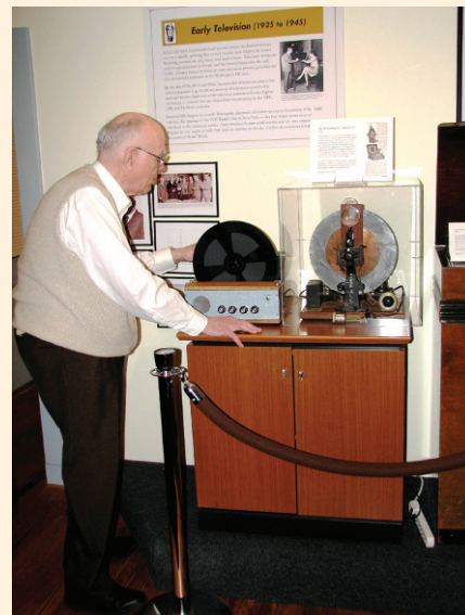
National Capitol Radio & Television Museum docent Noel Elliott demonstrates 28-line television circa 1928 with a specially crafted mechanical "televisor."
