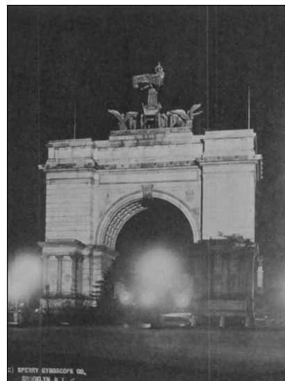
Photograph taken 2.5 mi from a High-Intensity Arc in the Sperry 60 in. Searchlight. An idea of the power and actinic value of the light may be obtained by comparing the dark lower right-hand portion of the arch which is illuminated by the street-lighting unit that is only 15 ft away from it. ( Fig. 3 from Trans. SMPE , Oct. 1920, p. 82.)
