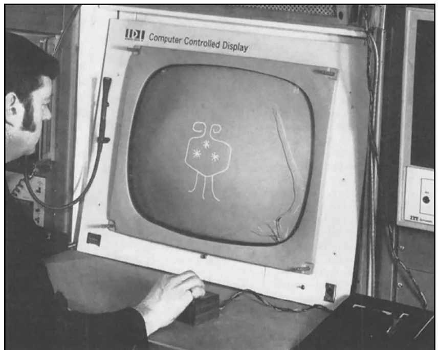
A handheld mouse being used for drawing. Also shown are thumbwheel encoders on right of the table, and the lightpen on the left of the CRT ( JSMPTE , Fig. 1, March 1971, p. 160).
