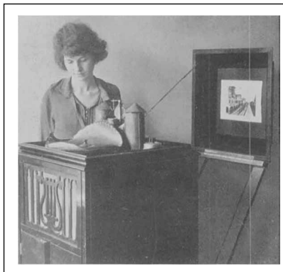
Discrola for Home Motion Picture Entertainment (Fig. 1 from Trans. of Society , May 1923, p. 234).
