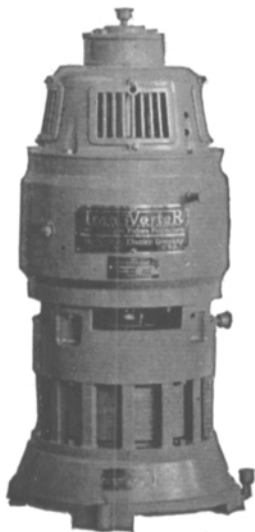
The A. C. to D. C. Transverter and Panel Board
